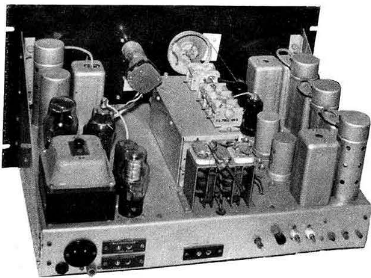
Rear view of the chassis. The tuning condensers are in the centre with the r.f./i.f. section to the right and a.f. and power supply stages on the left. Along the rear edge are the phone jack, mains input socket, send/receive jack, sockets for the loudspeaker field and output transformer, 5-meter sockets, and earth terminal. The stand-off insulators are for aerial input.
